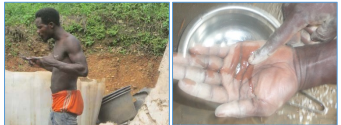
Figure 6. Miners Handling Gold Amalgam: On the left, a digger places gold amalgam in a metallic ladle with charcoal fire and fans it by blowing air with the mouth. On the right, a miner places mercury in the bare palm.
